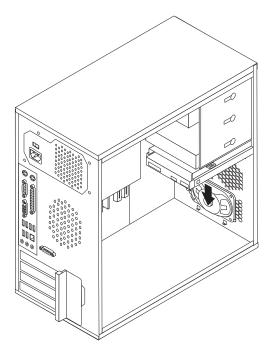
Figure 34. Installing a new internal speaker
